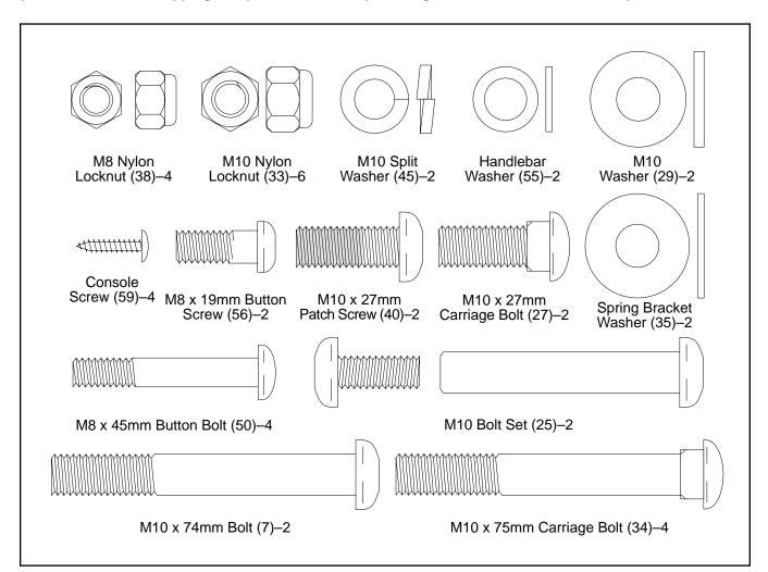
1. Identify the Front Stabilizer (10), which has round Endcaps (21) on it. While another person lifts the front of the Frame (1), attach the Front Stabilizer to the Frame with two M10 x 75mm Carriage Bolts (34) and two M10 Nylon Locknuts (33).
